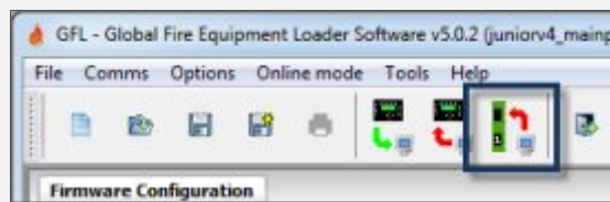
The toolbar button for sending the firmware, left of the exit button.
